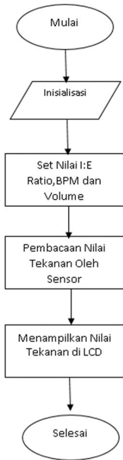
**Gambar 3. 5** Diagram Alir Sistem Tekanan Pada Ventilator
