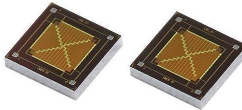
Gambar 2 Chip Thermopile
