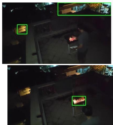
(a) (b) Figure 11. Sample of incorrect in detecting fire object (a) and sample of correct detecting fire object (b)
