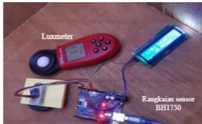
Gambar 4. 6. Proses kalibrasi sensor BH1750
