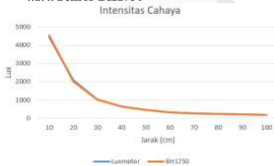
Gambar 4-7. Kalibrasi Sensor BH1750
