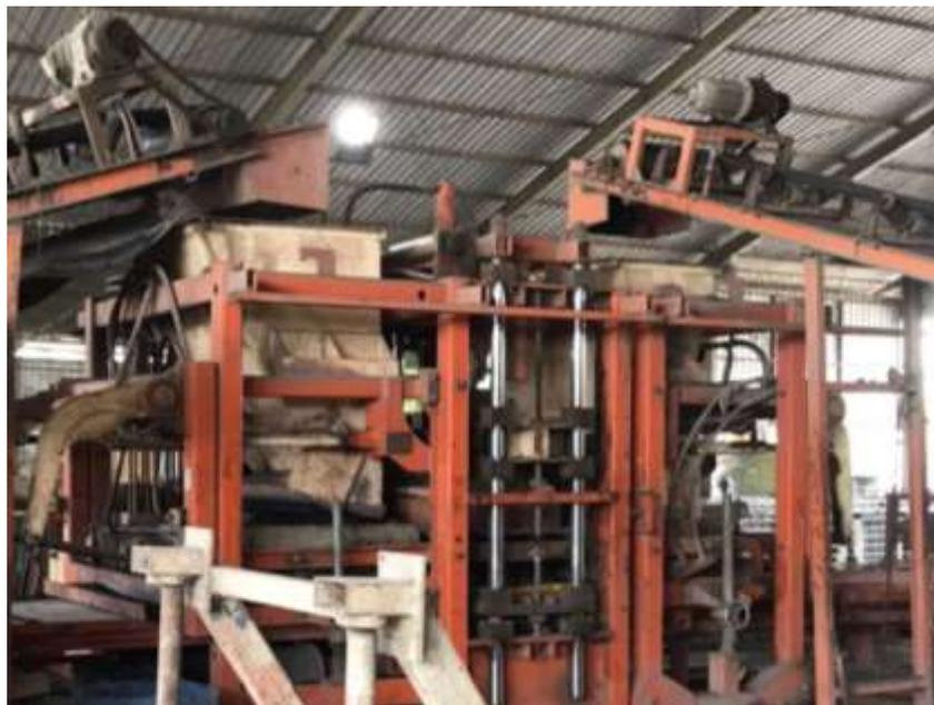
Gambar I 2 Mesin Pencetak Paving
