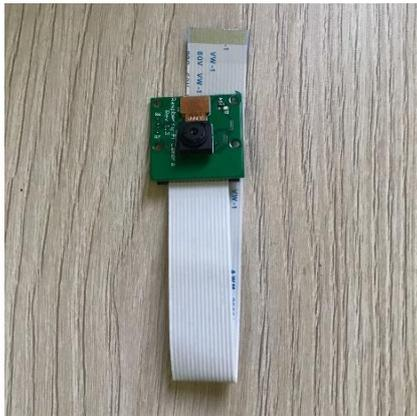
Gambar 2. Raspberry Pi Camera rev 1.3 5 MP
