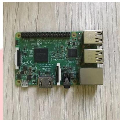
Gambar 3. Raspberry Pi model B V1.2
