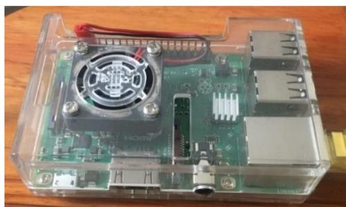
Gambar 1.1 Raspberry Pi Model 3B
