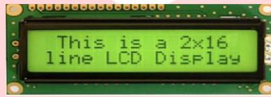
Gambar 2.9 LCD 16 x 02
