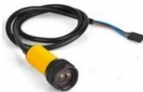
**Gambar 1** *Infrared Proximity Sensor* E18-D80NK
