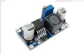
**Gambar 4** Modul *Step Down*
