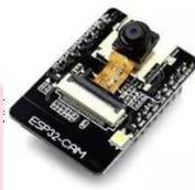
**Gambar 2** ESP32-Cam [8]
