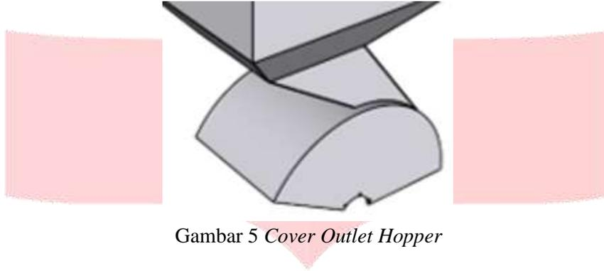
Gambar 5 Cover Outlet Hopper
