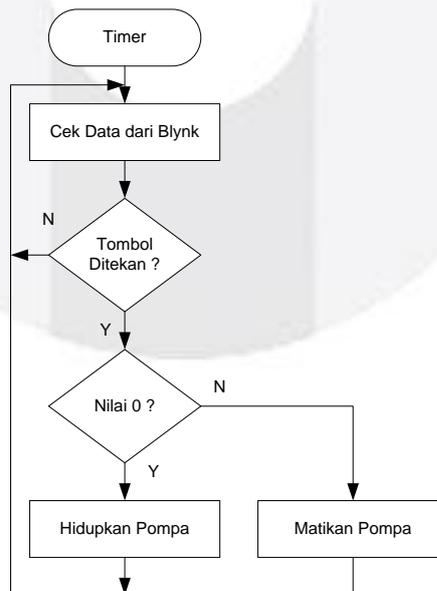
Gambar 3. Flowchart Penekanan Manual tombol on/off Pompa
