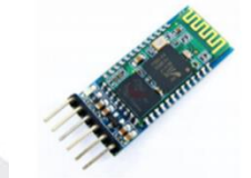
Gambar 7 Modul Bluetooth HC-05[11]
