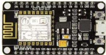
**Gambar 2.2** NodeMCU ESP8266 [10]
