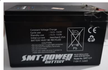
Gambar 3.5 Baterai 12V, 7.5AH
