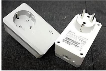
Gambar 1. Powerline Adapter AV600 TP – LINK
