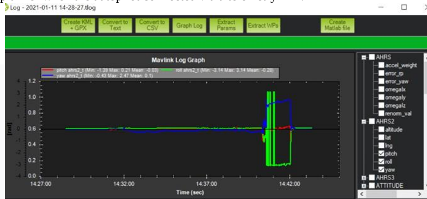
Fig. 8 - Graph of Stability drone in Mission Planner
