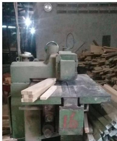
Gambar I.3 Mesin *Single Rip Saw*
