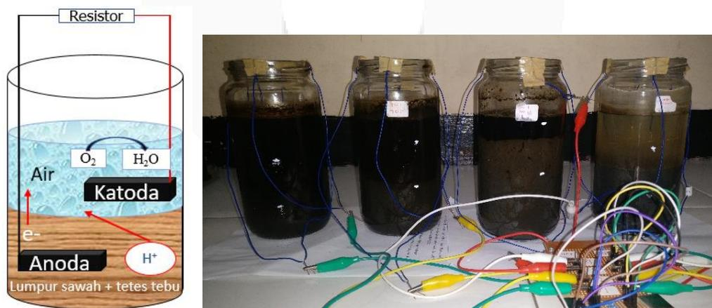
Gambar 2.1 Reaktor *single chamber* sistem SMFC.
