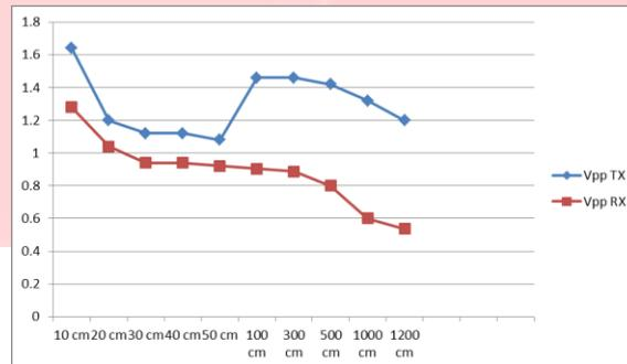
Gambar 6 Nilai Vpp Transmitter dan Receiver
