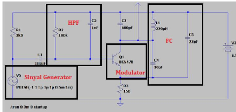
Gambar 2 Rangkaian Simulasi Transmitter FSK
