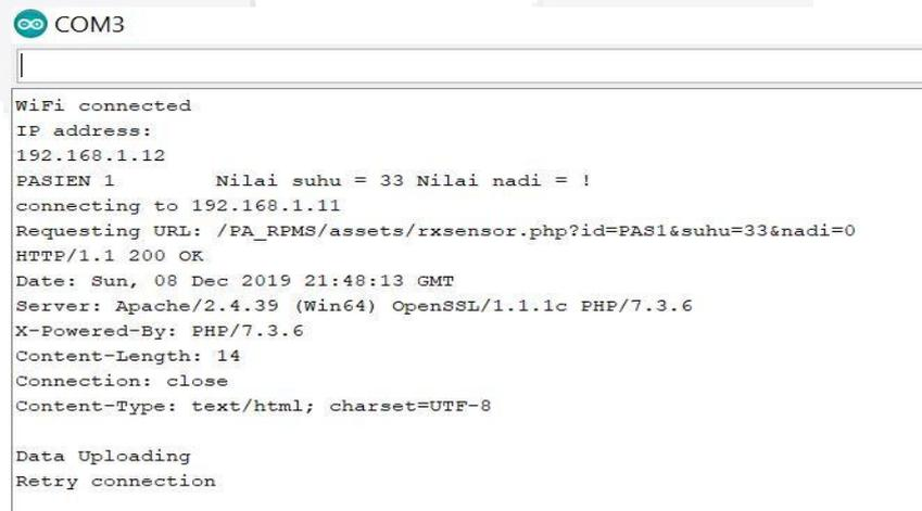
Gambar 3. 13 Upload data sensor ke database
