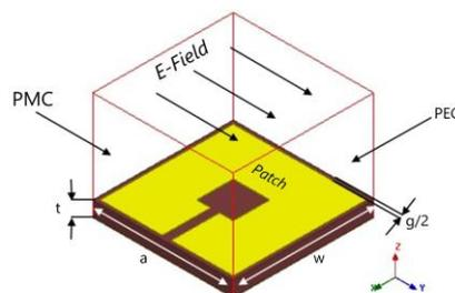
**Gambar 2.1** *Boundary* susunan *patch absorber*
