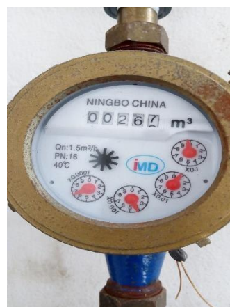
Figure 1.3 The water meter used is a Nutating type of Disk Meter (sumber: Indonesian watermeter)
