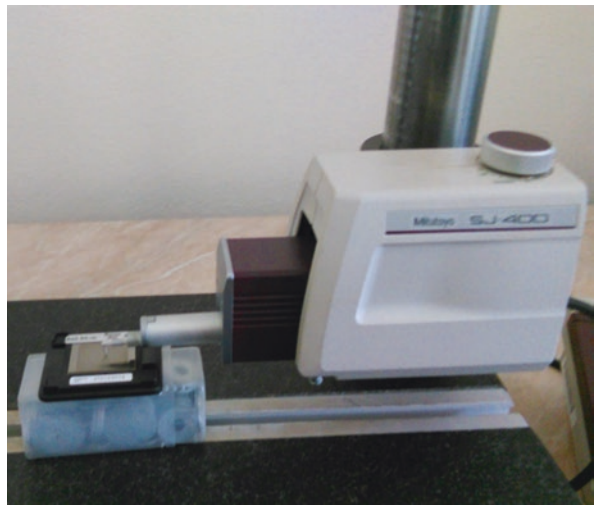
Fig. 26.7 Measurement a calibration sample on the measuring device Mitutoyo SJ 400
