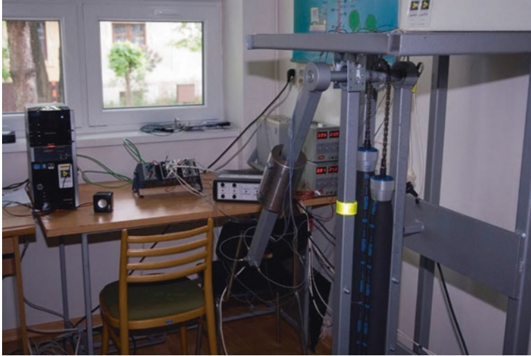
Fig. 4.3 Experimental device with drive based on PAM [7]
