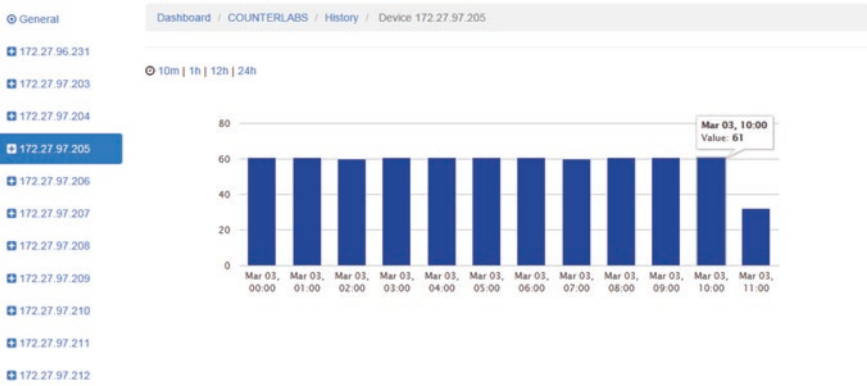
Fig. 7.8 Web graph visualization of performed mechanical cycles ( \times 100 ) for 12 h – displayed for one electronic counter IP module
