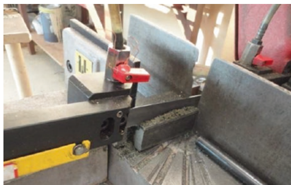
Fig. 25.1 Cutting of experimental samples on band saw
