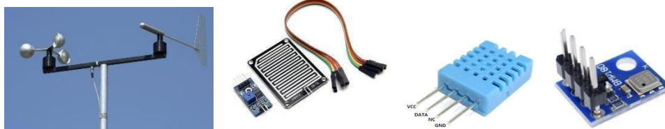
Gambar 2. Anemometer, Rain detector, DHT11, dan BMP180
