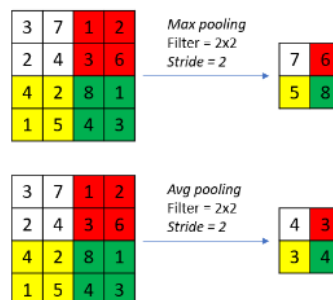
Gambar 4. Teknik max pooling (atas) dan average pooling (bawah)
