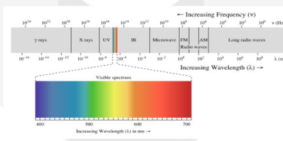
Gambar 2. 1 Elektromagnetic Spectrum.
