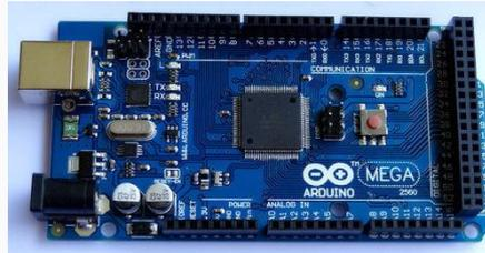
**Gambar 2.3** Arduino Mega 2560
