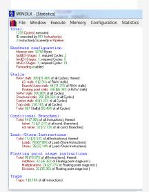
Figure 15. Statistics result of Haar DWT machine instruction.
