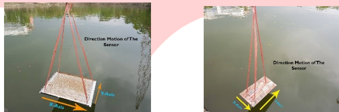
Figure 3.4 The Motion Direction of The Sensor. (a) Aluminium. (b) Ceramics
