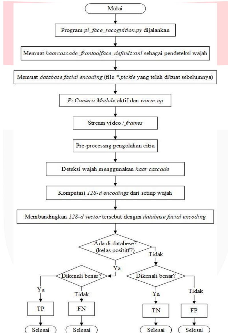
**Gambar 4:** Flowchart sistem *face recognition*
