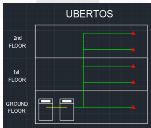
Gambar 3.7 Desain Denah Fiber to the Building Vertikal (Skenario 1)
