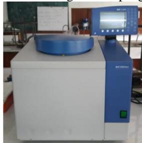
Gambar 1. Kalorimeter Bom IKA C2000 *Basic*.
