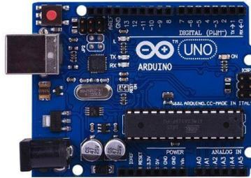
Gambar 2.2 Board Arduino UNO [11].
