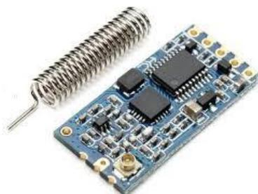
Gambar 2.3 Modul Transceiver HC-12
