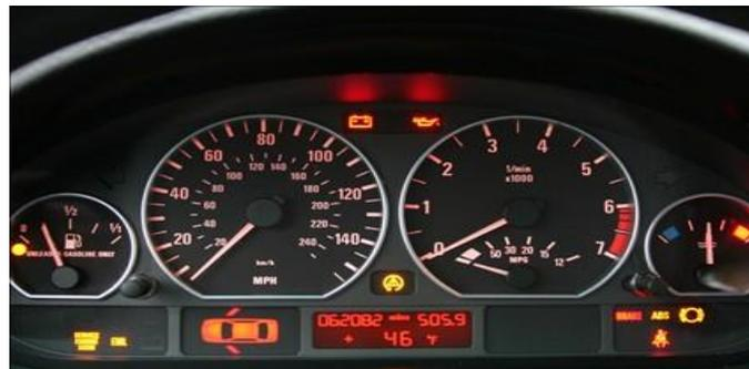
Gambar 2.2 Malfunction Indicator Light (MIL)
