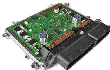
Gambar 2.1 Engine Control Unit (ECU)
