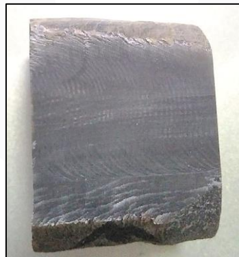
Figure 11 Workpiece used for measuring surface roughness
