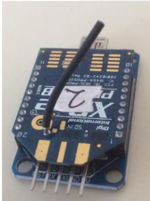
Gambar 2. 2 XBee Pro S2C
