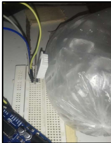
Gambar 4. 8 Pengujian batas minimum sensor DHT22
