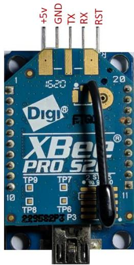
Gambar 2.6 Xbee pro s2c
