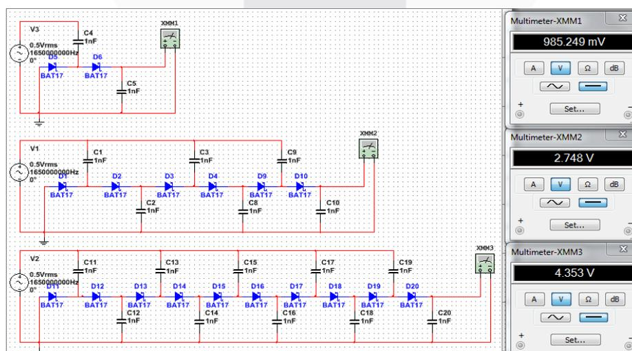
Gambar 7. Rangkaian *Voltage Doubler* 1 *stage*, 3 *stage*, dan 5 *stage*
