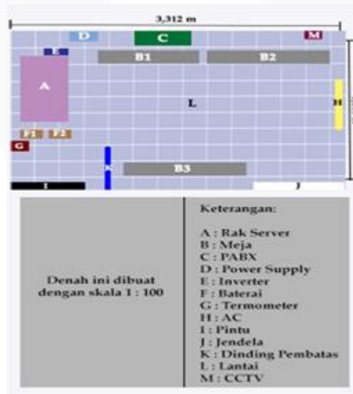
Gambar 4.2 Layout Ruang Data Center (Ruang Server)
