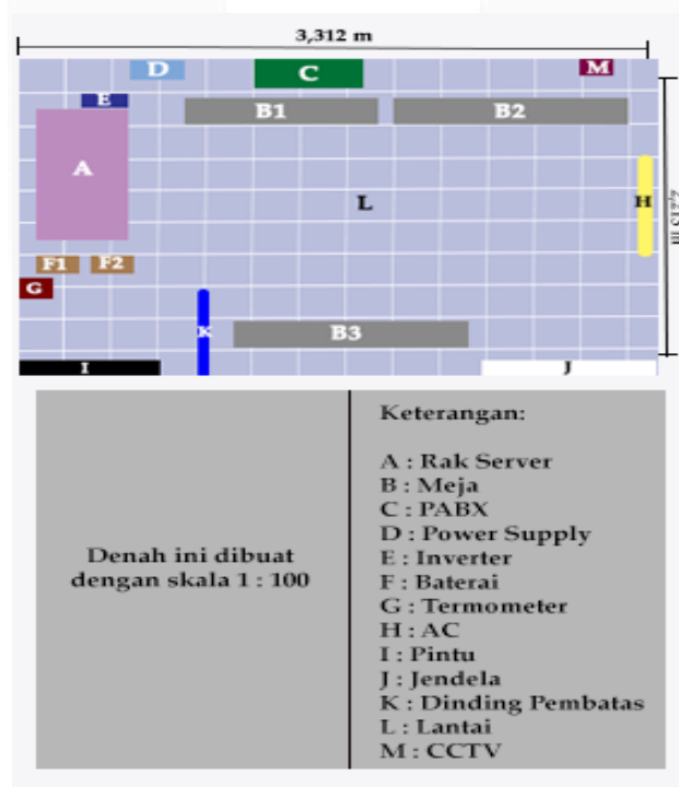
Gambar 3. Layout Ruang Data Center RSIM Sumberrejo
