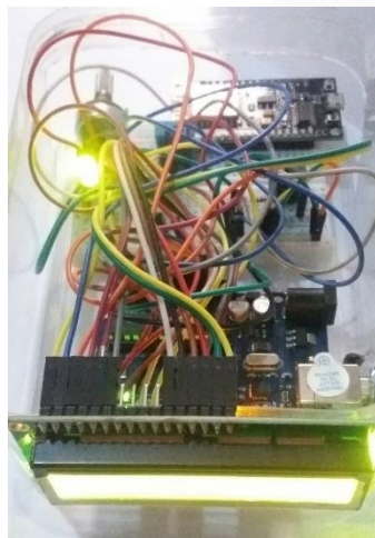
Gambar 7. Temperature Monitoring System Usulan Tier 2
