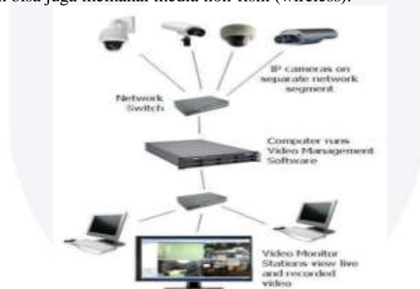
Gambar 2.2 Arsitektur IP-based Camera
