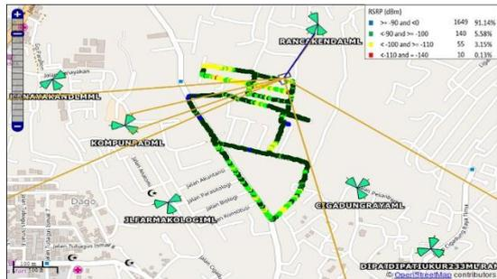
Gambar 4.4 Data Drive test After Coverage (RSRP) by MapInfo
