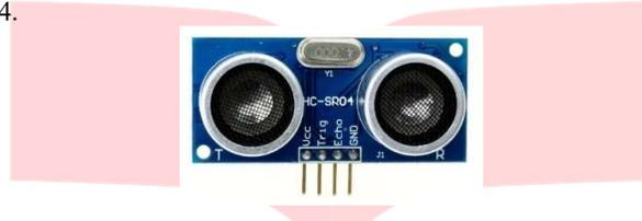
Figure 2. Sensor Ultrasonik HC-SR04
