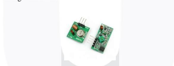
Figure 3. RF 433 MHz Trasmmitter dan Receiver
