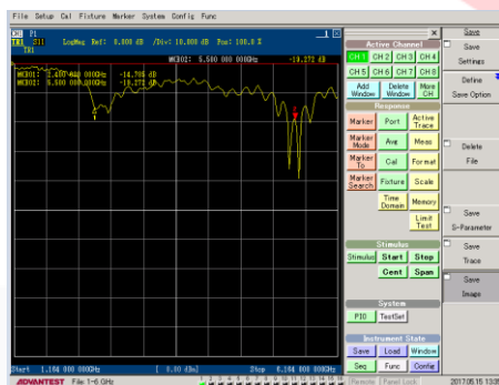
Gambar 4. 1 Pengukuran Return Loss
