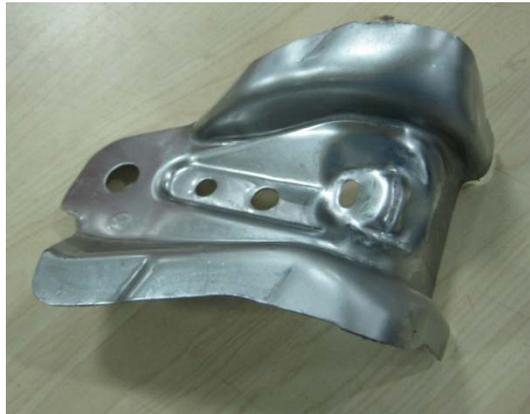
Gambar I.3 Gambar *Extension Floor Cross Rear Side*
