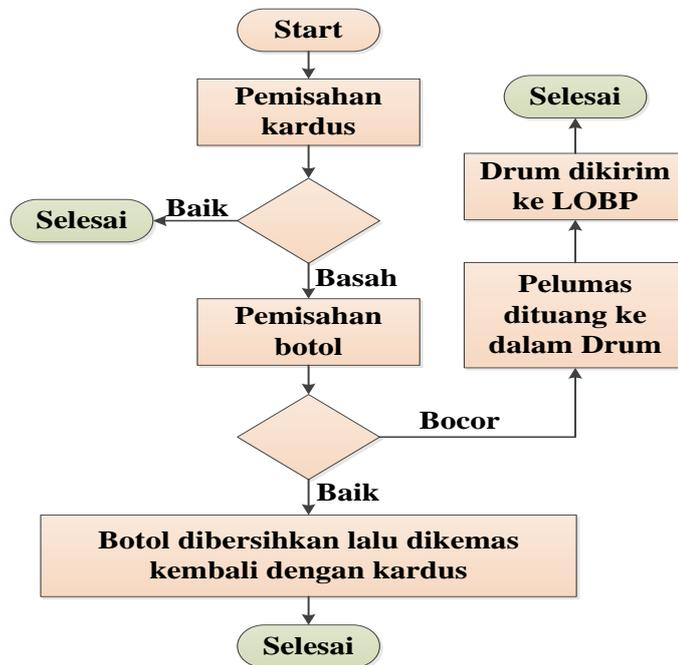
Gambar I. 2 Gambar Alur Proses *Repacking* Kemasan Kardus Basah
