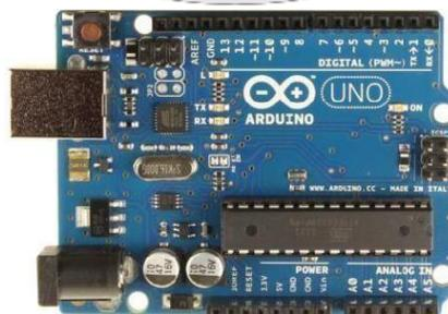
Gambar 2.5 Board Arduino Uno [11]
