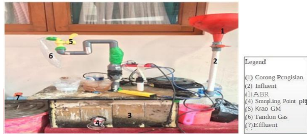
Gambar 3.1 ABR (Anaerobic Baffled Reactor) Semi Kontinyu
